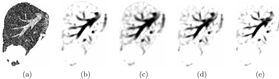
Fig. 2: (a) Image intensities (with lesion near bottom removed). (b) Maximum Flux . (c) Maximum CFlux . (d) Maximum MFlux . (e) Maximum SAMFlux .
